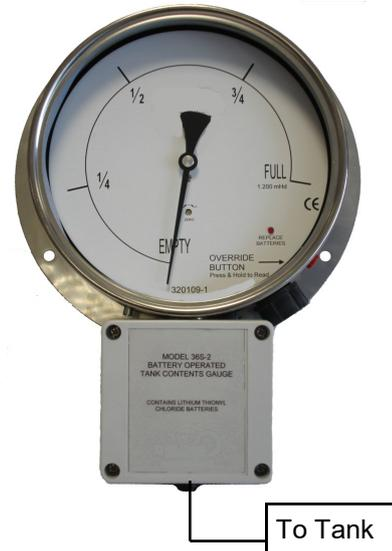
**RESET BUTTON** - In the unlikely event that you think the reading is incorrect, the reset button facility can be operated, this forces a reset of the timer system. When the button is pressed and released, the reading will rise then fall slightly, allow to settle, reading can now be taken. Once RESET has been used, **it cannot be re-used for a minimum of 30 mins**. Please note that this operation will dramatically reduce the battery life.
