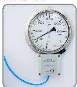
TEST LEVEL BUTTON - This is an override facility and can be operated at any time, if the button is pressed and held, the reading will rise then fall slightly, release button and allow to settle, reading can now be taken.
