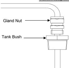
Suitable for tanks up to 8m deep, dependant upon SG, and liquids of viscosity up to 350 sec. Maximum remote indicator from tank 200m.
