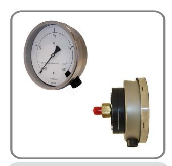
Specifically designed to measure water level in Sprinkler Tanks exposed to the freezing conditions. A bourdon tube pressure gauge will not function at below zero temperatures, the tube like any pipe that is filled with water will freeze and burst.
